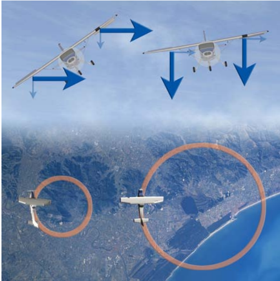
Figure 9: HORIZONTAL COMPONENT OF TIGHTER CIRCLES As ailerons are deflected, part of the vertical lift is diverted horizontally, thereby requiring additional power to maintain airspeed and altitude. The more the ailerons are deflected, the more lift is diverted and the tighter the airplane's turning radius becomes. The large arrows in this image show the balance of lift shifting from vertical (right) to horizontal (left). If the airplane were turned completely sideways ( 90^\circ bank), there would be no vertical lift left at all.
