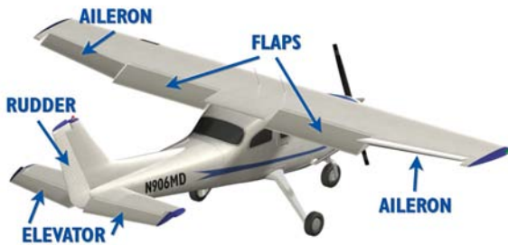
Figure 1: THE REAL AIR TRAFFIC CONTROLLERS Ailerons are controlled by turning the yoke left and right. They move opposite one another: as one goes up, the other goes down. Moving the yoke forward and back swings the elevator up and down. The rudder is controlled by the foot pedals and the flaps are either controlled by an electronic switch or a manual level, depending on the airplane model. The flaps, unlike the ailerons, move up and down in unison.
