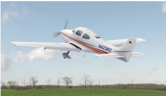
Figure 20: TAKING OFF SOFTLY This airplane has just departed from a grass airstrip (soft field) using partial flaps. The left (port) flap can be seen in this image just above the landing gear.
