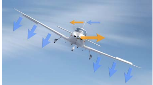
Figure 8: TURNING TAILS As the horizontal component of lift shoots off to the left (large blue arrows), sliding this airplane toward the right, the vertical stabilizer (tail section) hits the oncoming sideways airflow (small blue arrow) and resists the slide. The result is that the nose slides more and the airplane turns.
