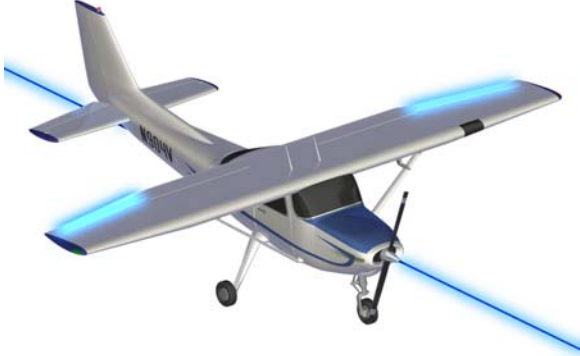
Figure 6: LONGITUDINAL AXIS Extending from the airplane's nose backward, is the longitudinal axis. The ailerons rotate the airplane around this imaginary line.
