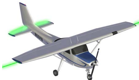
Figure 17: LATERAL AXIS Extending from wing tip to wing tip is the airplane's lateral axis. The elevator rotates the airplane around this axis to climb and descend. The absolute position of the lateral axis depends on the airplane's center of gravity, which varies from flight to flight.
