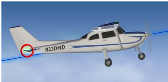
Figure 18: GOING DOWN? The elevator forces the tail section of the airplane up or down, which forces the nose oppositely. The rotation takes place around the airplane's lateral axis (the one that goes through the wings, not shown here), and realigns the airplane's longitudinal axis, shown here as a blue line.
