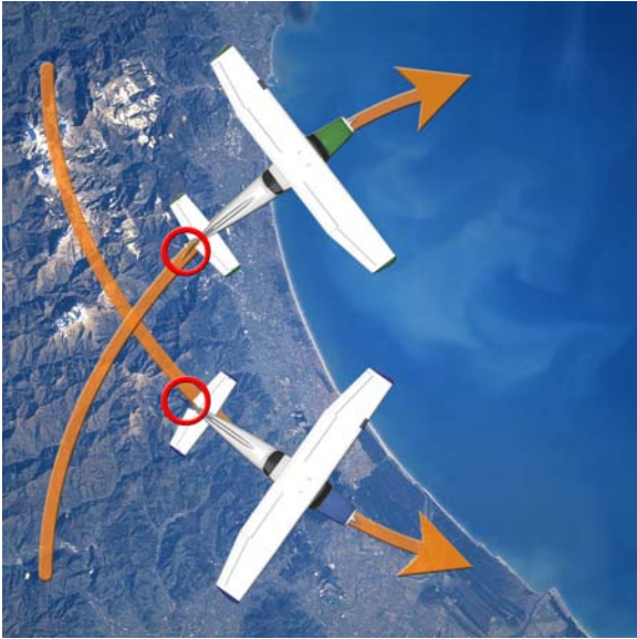
Figure 12: RIGHT RUDDER, MAYBE! The airplane's left-turning tendencies make the application of right rudder for the top airplane's right turn absolutely necessary. The pilot of the bottom airplane has applied no rudder pressure at all. The airplane's natural left-turning tendencies have aligned the longitudinal axis with the turn arc.
