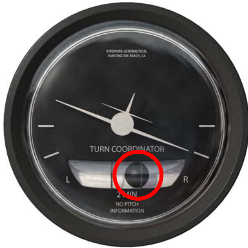
Figure 14: TURN COORDINATOR A turn is said to be coordinated when the ball (circled) remains centered throughout. In this image, the pilot must “step on the ball” with the right rudder to coordinate her turn. The airplane object is actually an indicator that tilts left and right. When level, it indicates the airplane is flying straight ahead. When the airplane’s wing tip aligns with the lower tick marks, the airplane is in a standard rate turn. The “2 MIN” indication on the dial tells us that a 360-degree turn at standard rate will take 2 minutes to complete, though the exact timing can vary somewhat for each airplane.
