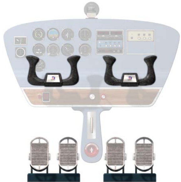
Figure 2: CONTROL SURFACE CONTROLLERS An airplane's yoke(s) and foot pedals are used to control the ailerons, elevator and rudder. The yoke rotates left and right like a steering wheel to control the ailerons, and forward and backward to control the elevator.
