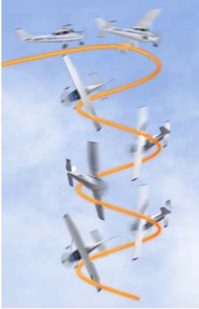
Figure 5: SPIN When one wing stalls before the other, it drops and the airplane might enter a spin. In this image the airplane's left wing stalled and dropped and the airplane entered the spin. This is the most common type of spin. Discuss spins and spin recovery with your CFI.
