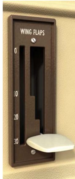
Figure 23: FLAP FLIPPER Most Cessna trainers have flap-position switches located toward the bottom of the instrument panel on the passenger side. The “stair stepped” position settings enable the pilot to choose flap settings by “feel” without having to actually look at the switch. Cessna aircraft have electrical motors that actually move the flaps; these switches control those motors. Piper flap levers look (and work) like parking brake levers found in some cars. As you pull up on the lever, the flaps deploy. Piper flap levers are physically connected to the flaps by rods and cables.
