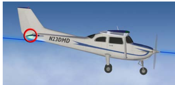
Figure 18: GOING DOWN? The elevator forces the tail section of the airplane up or down, which forces the nose oppositely. The rotation takes place around the airplane's lateral axis (the one that goes through the wings, not shown here), and realigns the airplane's longitudinal axis, shown here as a blue line.
