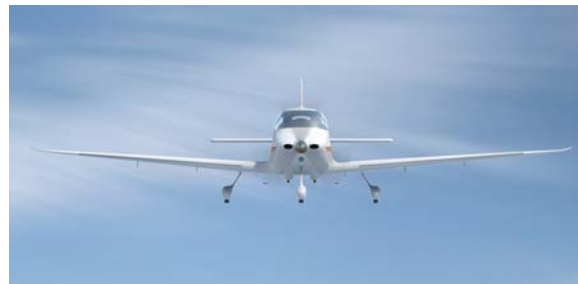
Figure 3: STRAIGHT AND LEVEL With no control surfaces deflected, this airplane flies straight and level. This configuration is also referred to as 'clean' because there is minimal interference with the relative wind.
