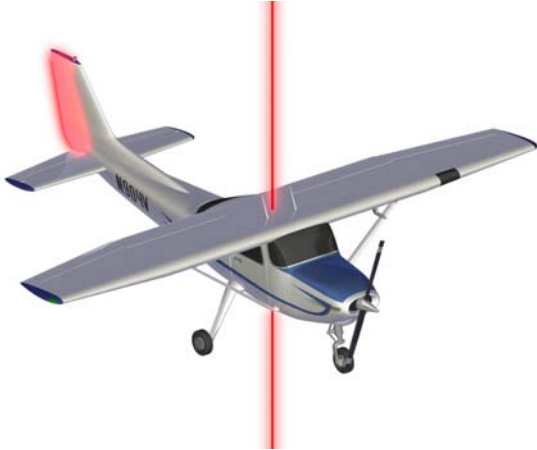
Figure 10: VERTICAL AXIS The rudder rotates the airplane around its vertical axis. This affects the airplane's attitude, but it does not, in and of itself, turn the airplane.
