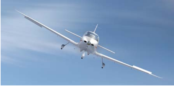
Figure 4: CONTROL SURFACE DEFLECTION The downward deflected right aileron (left) pushes the right wing up. The opposite happens on the other wing. Later we'll discuss how this turns the airplane.
