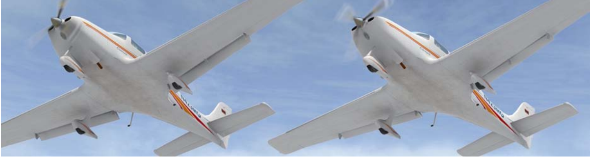
Figure 21: FUN WITH FLAPS Flaps increase lift and drag at the same time. The more the flaps are lowered, the more drag they introduce. Use of full flaps (left) enables an airplane to descend at a steeper angle without gaining airspeed. When flaps are lowered just a bit, say 10^\circ (right), they increase the wing's ability to generate lift without introducing too much drag. This flap configuration might be used when the airplane is taking off from a grass or dirt runway (what we call a soft field ) because the pilot wants to get the airplane out of the muck as soon as possible.
